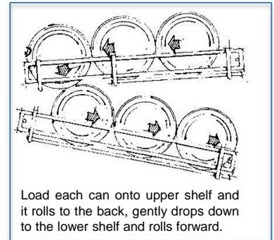
Load each can onto upper shelf and it rolls to the back, gently drops down to the lower shelf and rolls forward.
